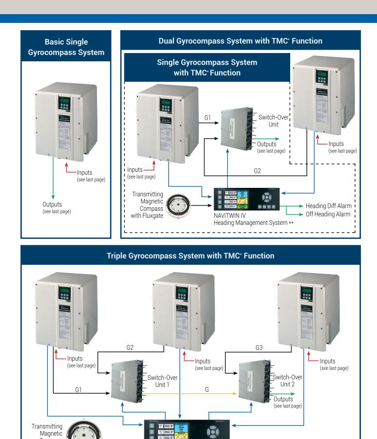
magnetic heading source for distribution to autopilots, repeaters, radars and other peripheral appliances when required. \*\* With selectable and programmable automatic heading takeover in accordance with Grounding Avoidance System (DNV NAUT OC and AW)
