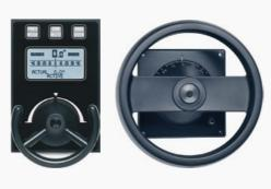
NAVIPILOT 4500N can be integrated with our versatile manual steering control system NAVIGUIDE 4000 that provides all required manual steering modes. NAVIGUIDE 4000 can be interfaced with a wide range of steering gears and can thus be adapted to customer needs.
